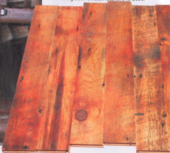
9 Cleared of nails, the wood is resawn and milled into boards for flooring and paneling.
